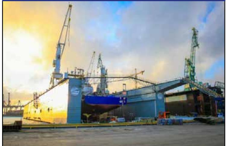
sludge, and electric motor overhaul, pipe replacement, bow thruster overhaul and complete hull treatment concluded with the application of anti-corrosive coating followed by two full coats of an anti-fouling coating.
